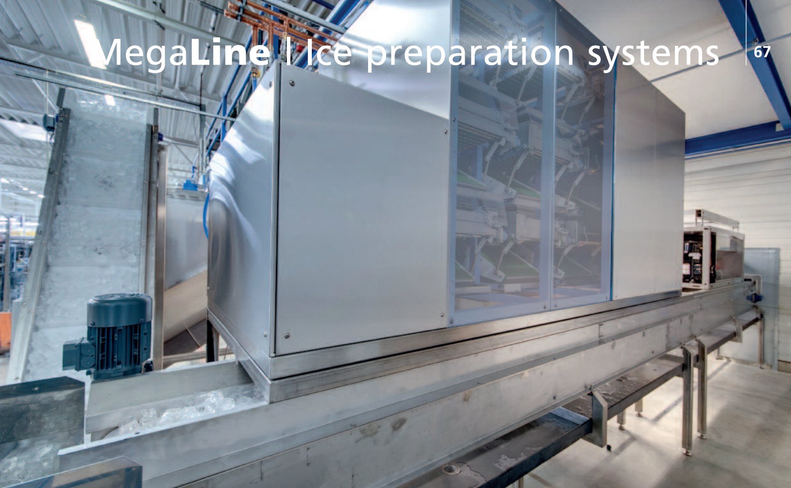
High-performance ice preparation plant IC 1500 with belt conveyor system and filling unit for square full ice cubes
