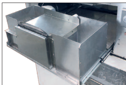
The extractable crusher unit facilitates the cleaning
