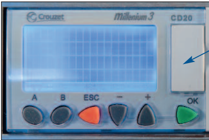
All models of the Micro-Cube ice makers are equipped with a reliable control (PLC). The current operating states are shown to the user via the digital display in the front panel.
