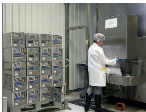
Ice production with semi-automatic filling of hollow ice cones for the inflight catering
