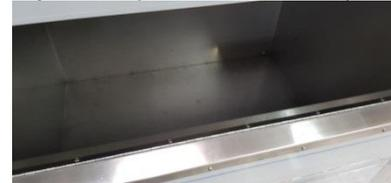
3. Thoroughly rub all storage container walls with a cloth soaked in WESSAMAT special cleaner so that all dirt and limescale residues are removed. Rub thoroughly with clear water to remove all cleaner residues.
